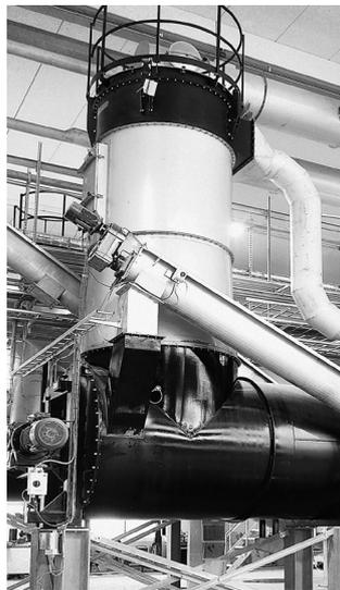
This sturdy, no-frills cooler enables you to use ambient air to cool a broad range of meal products (usually derived from poultry, fish or meat) after they have passed through a dryer. Cooling helps make the processed cake more brittle, so it's easier to mill.
