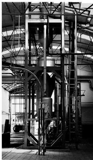
If you need to process feathers or hog hair into a high-quality feed meal that contains a minimum of indigestible proteins, the Haarslev Vertical Hydrolyzer is an extremely effective way to do it.
