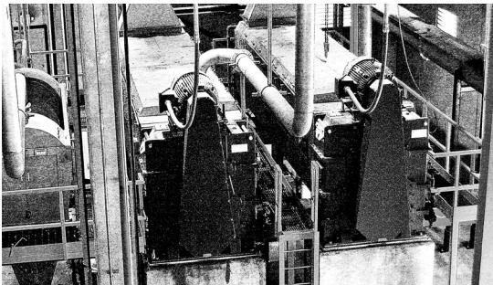
A Haarslev Twin-screw Press is ideal for extracting liquid from cooked fish or meat as part of wet rendering processes. These units provide you with an effective way to remove water from the fats and solids content in cooked fish or meat. This then helps you improve the overall efficiency of subsequent processing and paves the way to significant energy savings.
