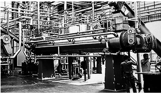
Rugged, energy-efficient Haarslev screw cookers are ideal for processing setups where inputs vary in both quality and composition, with a bare minimum of pre-cooking preparation. You can choose throughputs from 2 to 50 metric tons per hour, and the modulating valve for the steam supply makes it easy to process even small volumes if and when needed.
