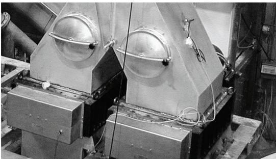
Smaller, more consistent particle sizes are an effective path to better efficiency in a wide range of meat and poultry processing setups. Smaller particles make heating processes more cost-effective and energy-efficient, making Haarslev Fine Crushers a valuable addition to processing lines that focus on operating costs.
