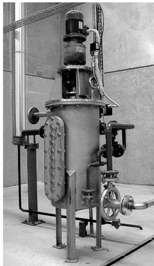
This is a simple, durable setup that helps boost the effectiveness of a wide range of animal and poultry blood treatment processes by making the solids component coagulate so it's easier to remove the water content.
