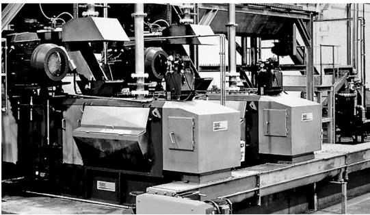
The Haarslev Fat Screw Press provides highly effective mechanical extraction of the fat content from cooked and dried animal and poultry by-products, in a continuous flow. This enables you to achieve a hard cake with a low fat content.
