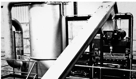
The Haarslev Milling Plant effectively reduces the size of particles in the not-yet-finished meal after fat extraction, helping you meet customer specifications about particle size.
