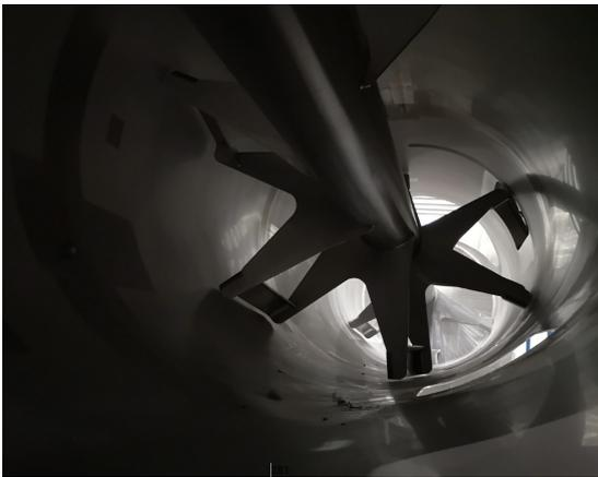
This robust, hard-wearing cooler enables you to use ambient air to cool a broad range of meal products (usually derived from poultry, fish or meat) after they have passed through a drying or cooking process. Cooling helps make the processed cake more brittle, so it's easier to mill.
