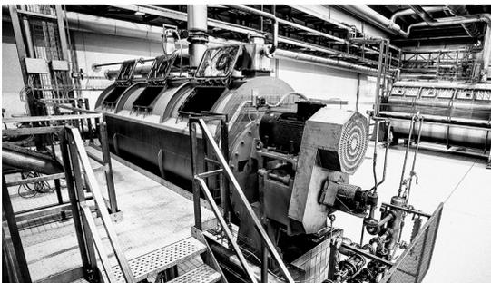
The Haarslev Coil Dryer is the ideal solution for the continuous drying of free-flowing, semi-dry, low-fat, inputs that include fish meal, blood and feathers.
