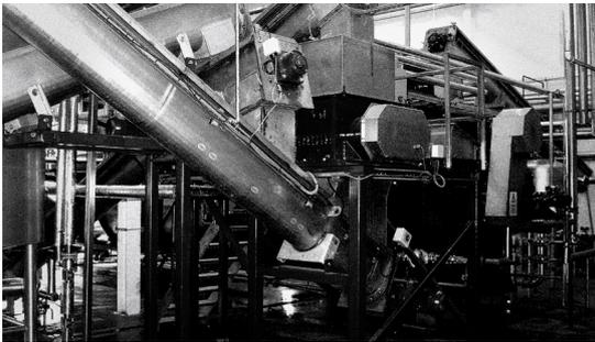
The Haarslev Screw Conveyor is specially designed to help you move material from one step to the next in your processing setup, coping easily with often-considerable height differences by operating reliably with an incline of as much as 30 degrees. This helps ensure processing continuity and higher overall outputs, by eliminating bottlenecks and “weak links” between the efficiency of individual processes.
