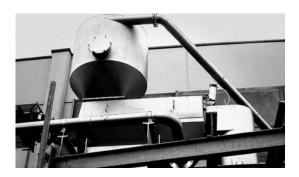
FOR REMOVING WATER FROM THE HOG HAIR FROM SLAUGHTER LINES. The Haarslev Hog Hair Press enables you to drastically reduce the amount of water in batches of hog hair. This can reduce weight by as much as 50%.
