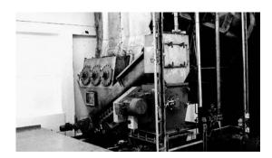
STRAIGHTFORWARD, HIGH-SPEED CRUSHER FOR ALL KINDS OF HARD OR SOFT ANIMAL OR FISH BY-PRODUCTS. The Haarslev High-speed Crusher enables you to effectively, continuously crush almost any kind of animal or fish byproducts, hard or soft. Models are available for production flows of 2–25 tons/hour (or more).
