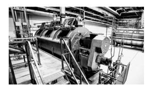
FOR CONTINUOUS DRYING OF LOW-FAT. NON-STICKY PRODUCTS SUCH AS FISH MEAL, BLOOD AND FEATHERS. The Haarslev Coil Dryer is the ideal solution for the continuous drying of free-flowing, semi-dry, low-fat, inputs that include fish meal, blood and feathers.
