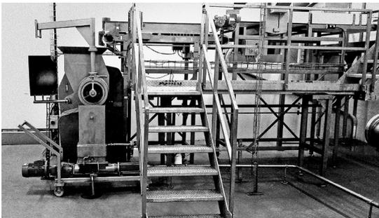
Haarslev Hopper-fed Grinders are reliable, larger-capacity units that are ideal for grinding fine or coarse, fresh or frozen animal by-products, prior to further processing in which consistent particle size helps increase efficiency.
