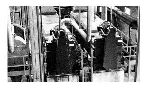
A Haarslev Twin-screw Press is ideal for extracting liquid from cooked fish or meat as part of wet rendering processes. These units provide you with an effective way to remove water from the fats and solids content in cooked fish or meat. This then helps you improve the overall efficiency of subsequent processing and paves the way to significant energy savings.
