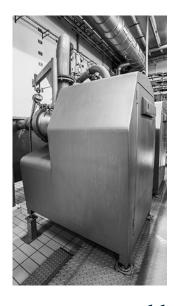
HIGH-CAPACITY PUMP-FED GRINDER FOR REDUCING PARTICLE SIZE IN RELATIVELY, SOFT VISCOUS ANIMAL BY-PRODUCTS. The Haarslev Pump-fed Grinder performs particularly well with softer viscous, pumpable inputs. The connected feed pump ensures a consistent flow rate that helps eliminate slippage. The consistent flow also ensures clean cutting of the material passing through the grinder, and outputs in best possible condition.
