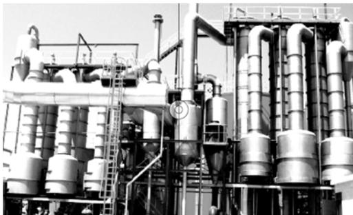
The most widely used Haarslev evaporators use the falling-film principle to concentrate these liquids, drawing thermal energy from the dryer in order to bring the liquid up to temperatures at which the water content evaporates. This means you can achieve higher concentrations at lower cost, and also recover the dissolved higher-protein solids to boost yields in your meal production setup.
